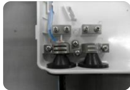
2. Insert fiber cable into the input holes, then fix it on the box by suitable fixation clamps as picture. (The length of input cable about 1M )
